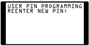
4. To confirm your entry, reenter the PIN number you just entered in step 4 above + **HOLD**. At a 22- or 34-Button Display Telephone, you see:
