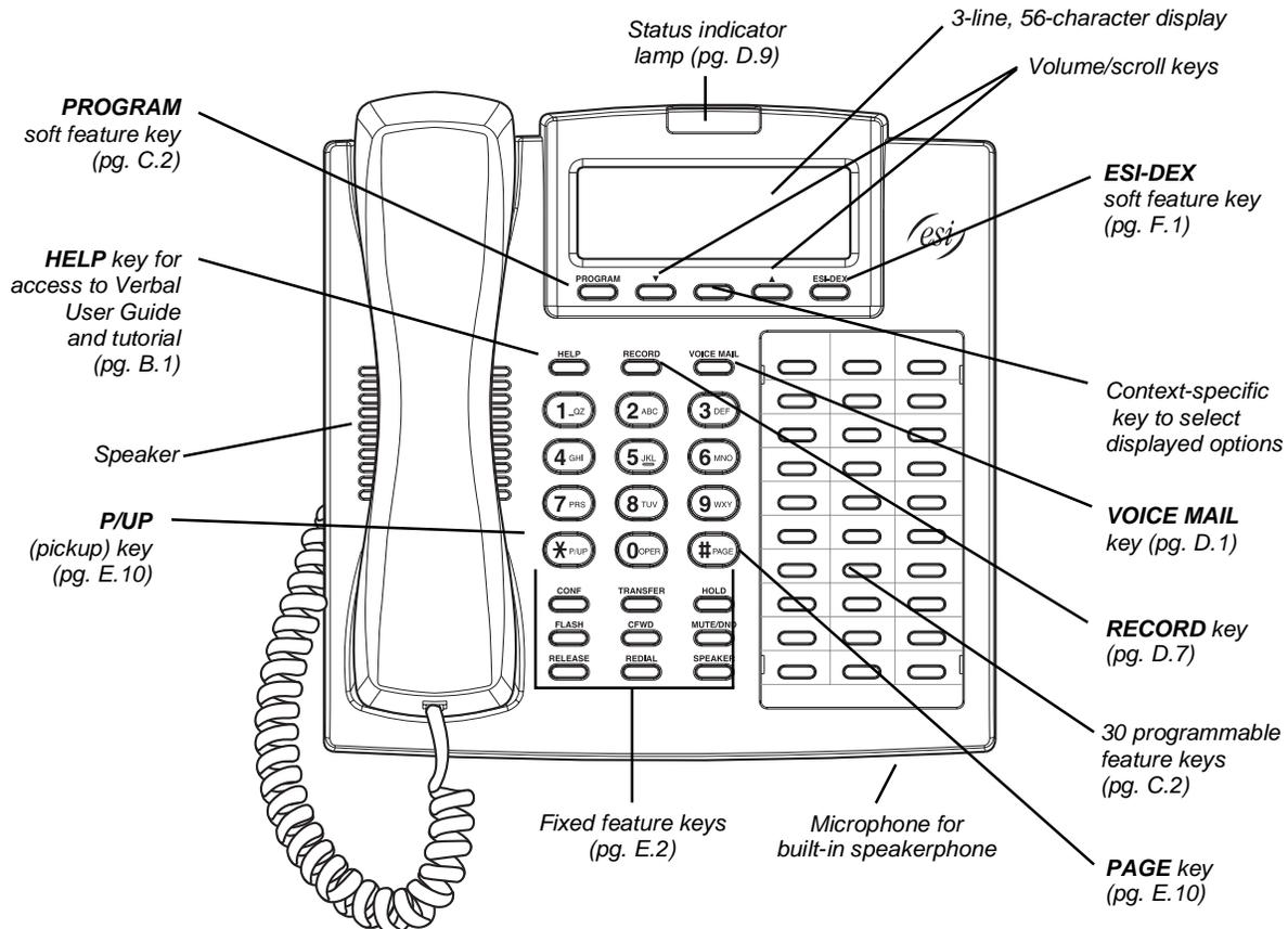
**Hint:** On any of these phone varieties (including the 60-Key Expansion Console), you can perform **direct programming** by holding down a programmable feature key for at least two seconds (similar to how you might program a car radio button). This isn't applicable to the fixed-feature keys which, as their name implies, are already programmed.
