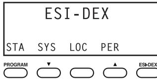
2. Press a key to choose the appropriate Dex —Station Dex (**STA**), System Dex (**SYS**), Location Dex (**LOC**) or Personal Dex (**PER**) — or press **RELEASE** to cancel the procedure.
