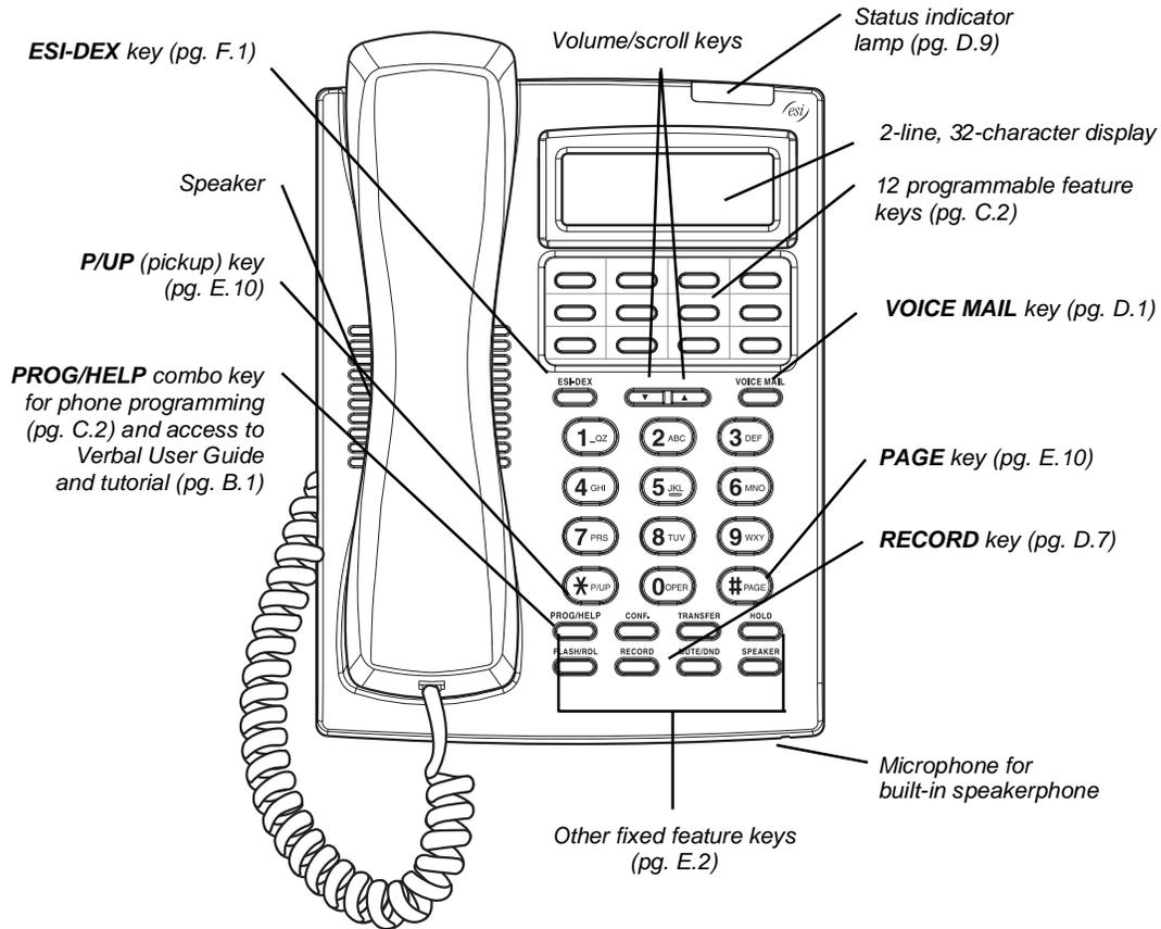
**Hint:** On any of these phone varieties (including the 60-Key Expansion Console), you can perform **direct programming** by holding down a programmable feature key for at least two seconds (similar to how you might program a car radio button). This isn't applicable to the fixed-feature keys which, as their name implies, are already programmed.
