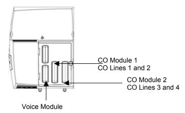
6B: Installing CO Modules in the Extension module
