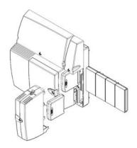
**NOTE:** Ensure all the locking screws are locked after the modules are installed.
