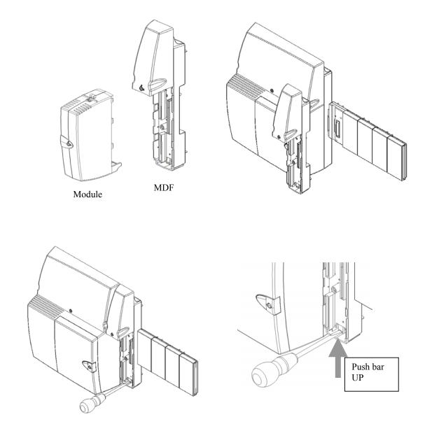
Push the Locking bar UP to lock the MDF in place
