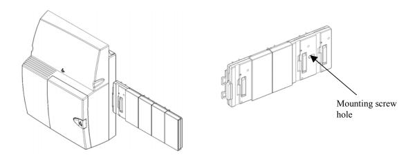
IMPORTANT: The backplane must be secured to the wall bracket using the mounting screw to ensure it is securely locked in place and does not move when modules are being installed.
