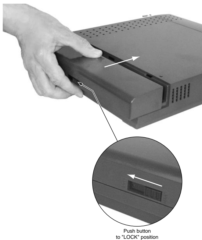
Figure 3-5: Reinstalling the Cover
